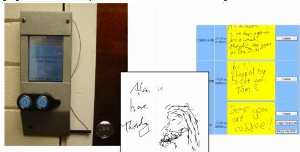
Hermes unit with note from door owner and web interface viewing notes left by visitors
